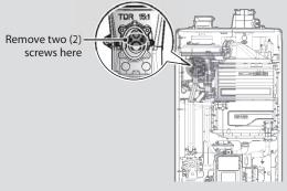
Figure 4. Access to Gas Orifice in Fan Assembly
