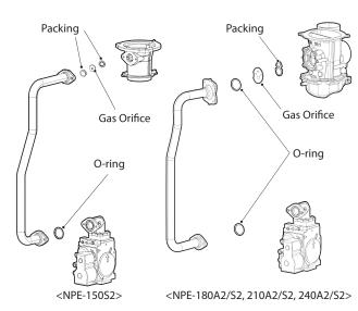
Figure 5. Exploded view of Gas assembly
