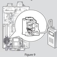
b. Connect a manometer to the offset pressure port. For dual port manometers, use the positive pressure side.
