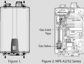
NPE-A2/S2 Series Front cover Internal Components
